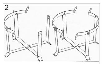
Insert two screws to attach one cart band to the legs. Insert the screws from the inside of the cart, and tighten the acorn nuts on the outside by hand. Repeat this step to attach the other band.
