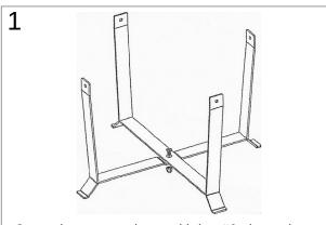
Cross the two cart legs, with leg #2 above the other. Insert the screw from the top, and tighten the acorn nut on the bottom by hand.
