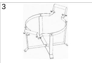
Attach the two handles to the cart using a screwdriver. Then tighten all of the nuts with the included wrench.
